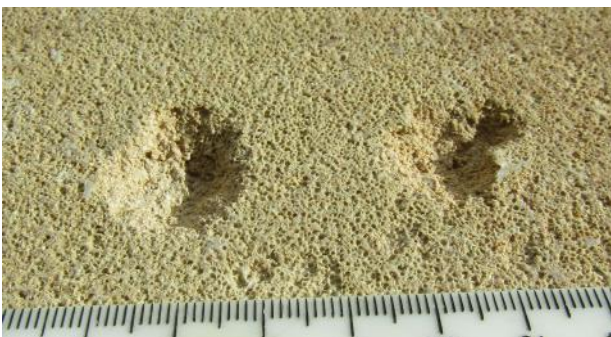
Fig. 16: Ballistic impact marks (scale in mm) in Bath Stone from an air-rifle using .177 calibre Webley VMX pellets from a distance of 2 metres. These mini-craters are similar to some of those on buildings in Bath.
