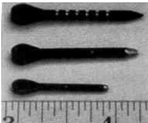
Fig. 15: Flechettes – aerial darts dropped by planes, are the correct size for the small impact marks with central holes. Scale inches. Image: Wikimedia Commons.
