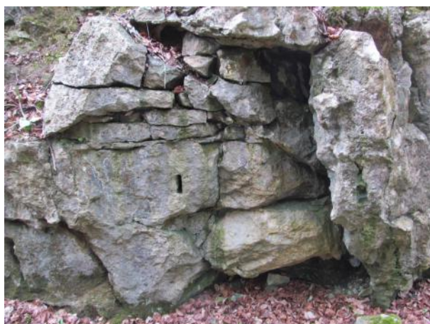
Fig. 7: Bolt hole in Bath oolite in an old quarry at Brown's Folly, Bathford; dimensions are 10 x 2 cm.
