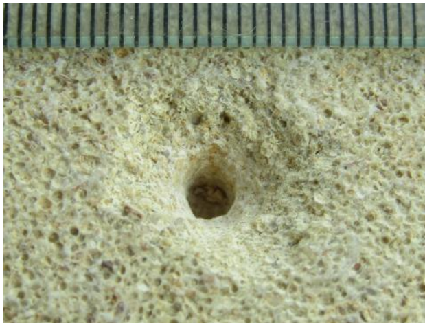
Fig. 18: Hole created from the impact of hammering a nail into a block of Bath Stone. Scale mm.
