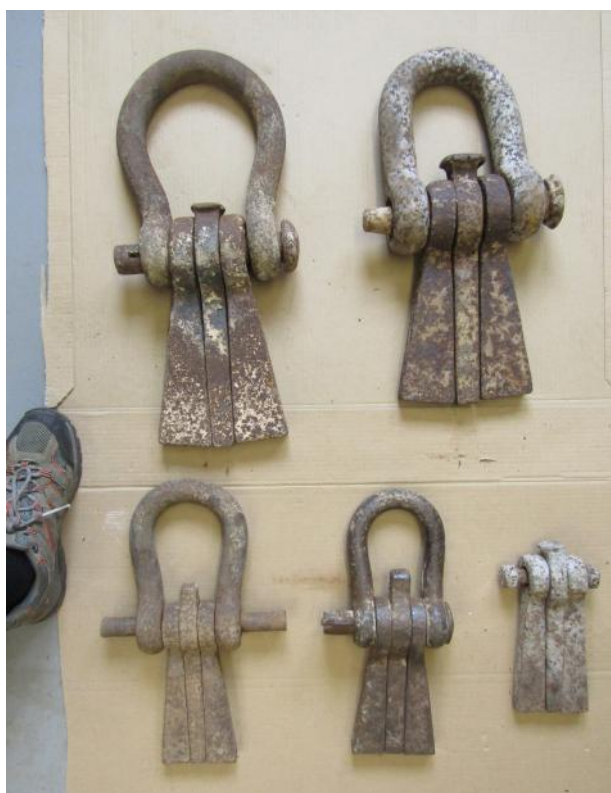
Fig. 1: Five lewis bolts from David Pollard's collection from the Box-Corsham mines. The total length of the largest (top left) is 53 cm.
