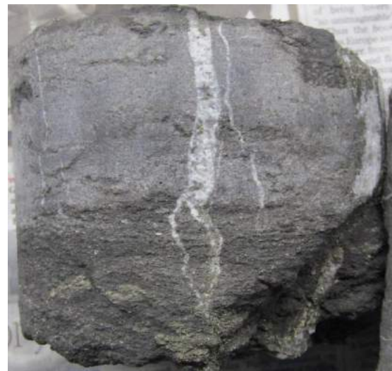
Figure 5. Core of thin limestone bed with a cm-wide fracture (Core 8 cm across.)
