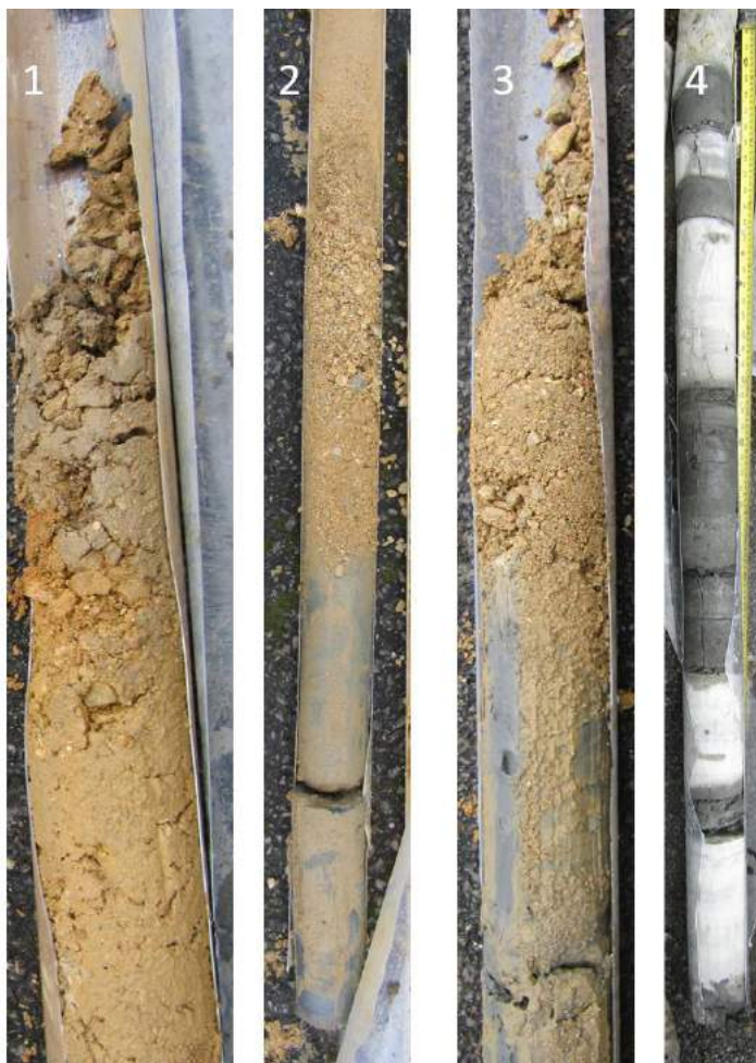
Figure 1. Example of the cores recovered from recent drilling at a planned building site by the River Avon in Bath.
