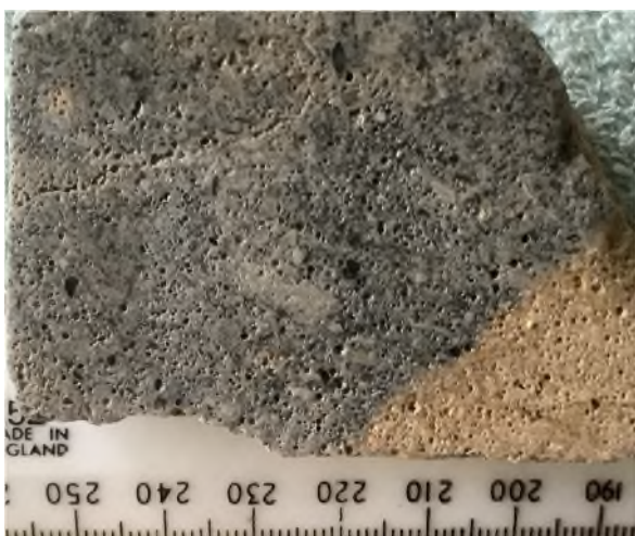
Figure 2. Cut surface of a blue-coloured sample of Bath stone with a sharp boundary to the more typical honey-coloured stone.
