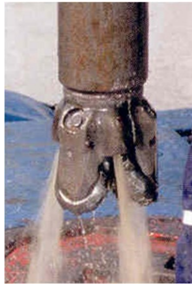
Figure 4: Use of drill bit nozzle in jetting and whipstock. Both used to initiate a directional well
