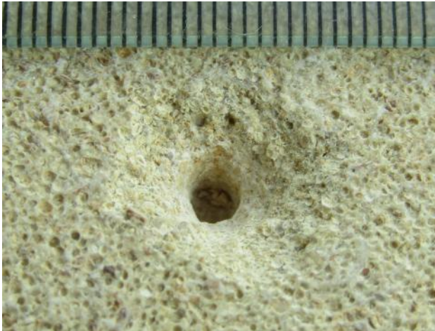
Fig. 18: Hole created from the impact of hammering a nail into a block of Bath Stone. Scale mm.
