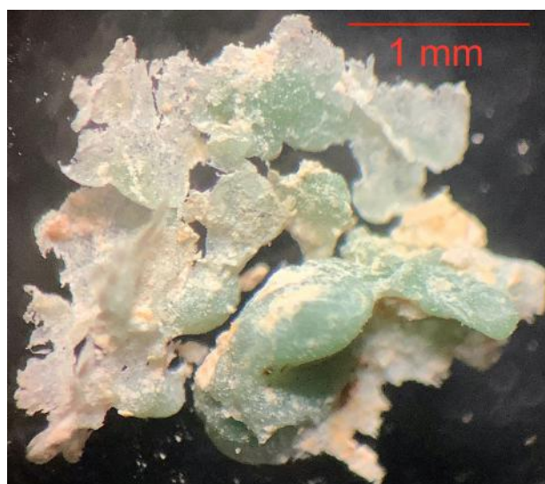
Fig. 6: Green and flaky grains extracted from Bath oolite interpreted as glaucanite. Our experiments focused on the largest grain at the bottom right of this image.
