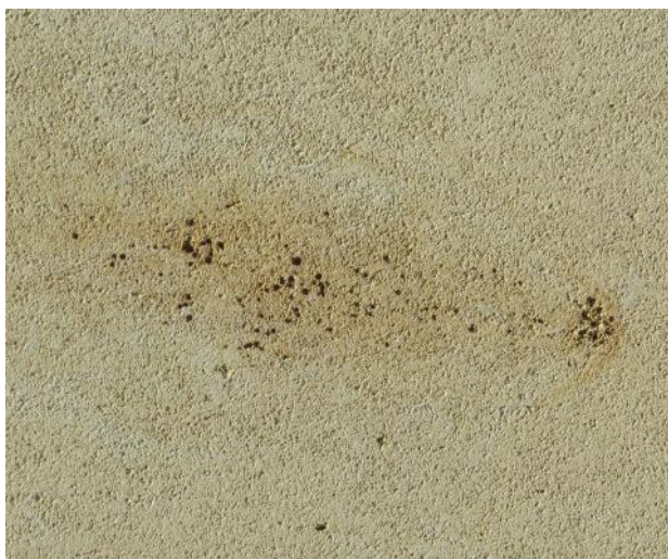
Fig. 3: Orange-brown stain emanating from rusting pyrite crystals and spreading out into the oolitic limestone. Field of view 15 cm across.
