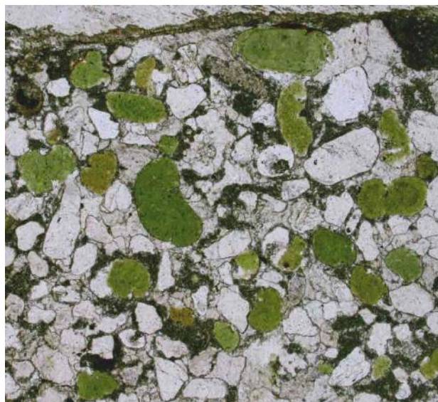
Fig. 4: Photomicrograph of glaucanite grains along with quartz grains in Greensand, Dorset. Plane polarised light. Field of view 8 mm across.
