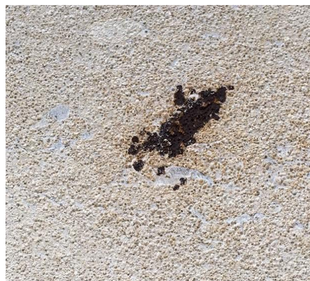
Fig. 1b: An elongate nodule of pyrite crystals, likely formed within a burrow. Field of view 6 cm. Bath Stone, Bath Riverside.
