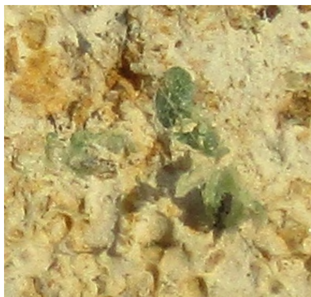
Fig. 5: Close-up of glaucanite grains in Bath oolite. Field of view 8 mm across.
